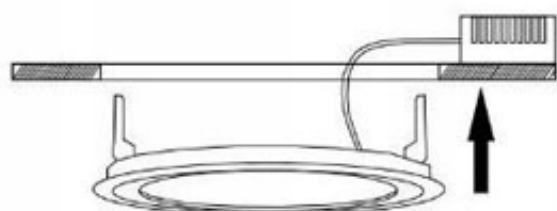
(3) built-in the panel to the ceiling
